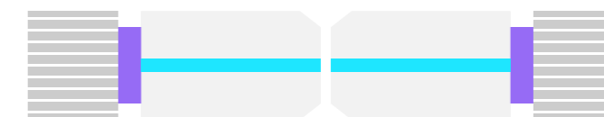
Ultra Physical Contact Connector
