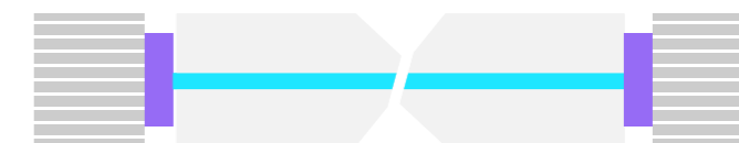
Angled Physical Contact Connector
