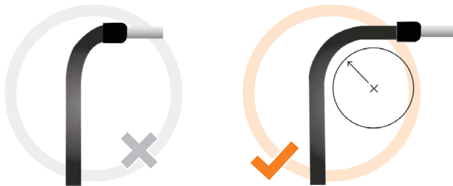
Risk of breakage due to overload
