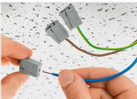
To connect: Insert stripped solid conductor into circular entry and push until it hits the backstop.
