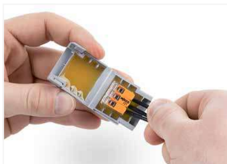
Place the wired connector in the Gelbox.
