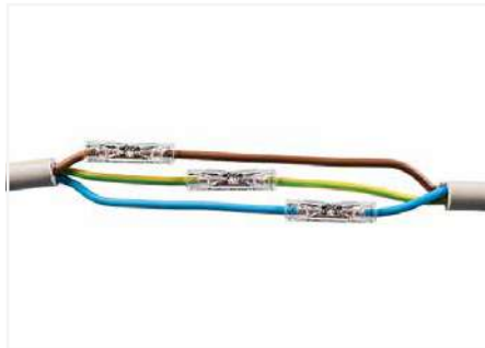
Strip 10 mm conductor per specification and insert connector (example shows staggered connectors).
